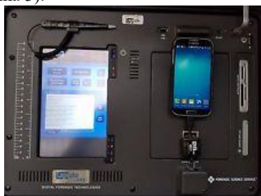
Slika 3 LOGICUBE CellDek F-LC7000 Police Forensic Cell Phone Data Extraction Analyzer
